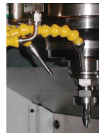
Pinpoint control of Micro-Droplets eliminates hazardous misting
