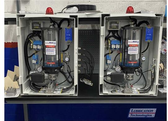
Each Pump Package consists of an 8 kg high pressure (4,300 psi) pump delivering lubricant to a master divider valve in the enclosure. The configuration provides for both low level lubricant as well as no flow lubricant status indication via digital read out on the face of the controller as well as a strobe light which would notify personnel in the event of either condition.
