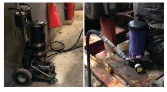
Use of Harvard Portable Filter Cart dramatically reduces particle count as evidenced
