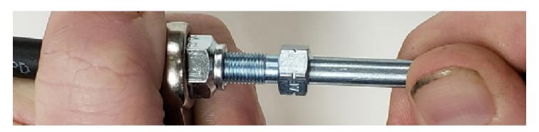
Use a 10mm wrench to tighten the hose stud to the sleeve, in a clockwise motion.
