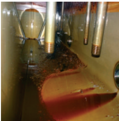
Figure 1 The formation of both sludge and varnish in a hydraulic oil reservoir
